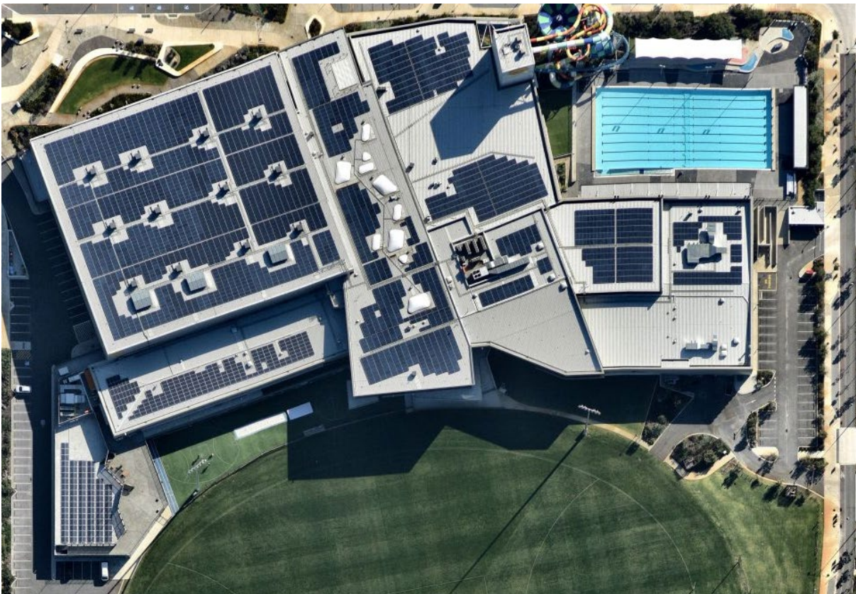
Figure 8: Cockburn ARC, showing the existing 1 MW solar system
