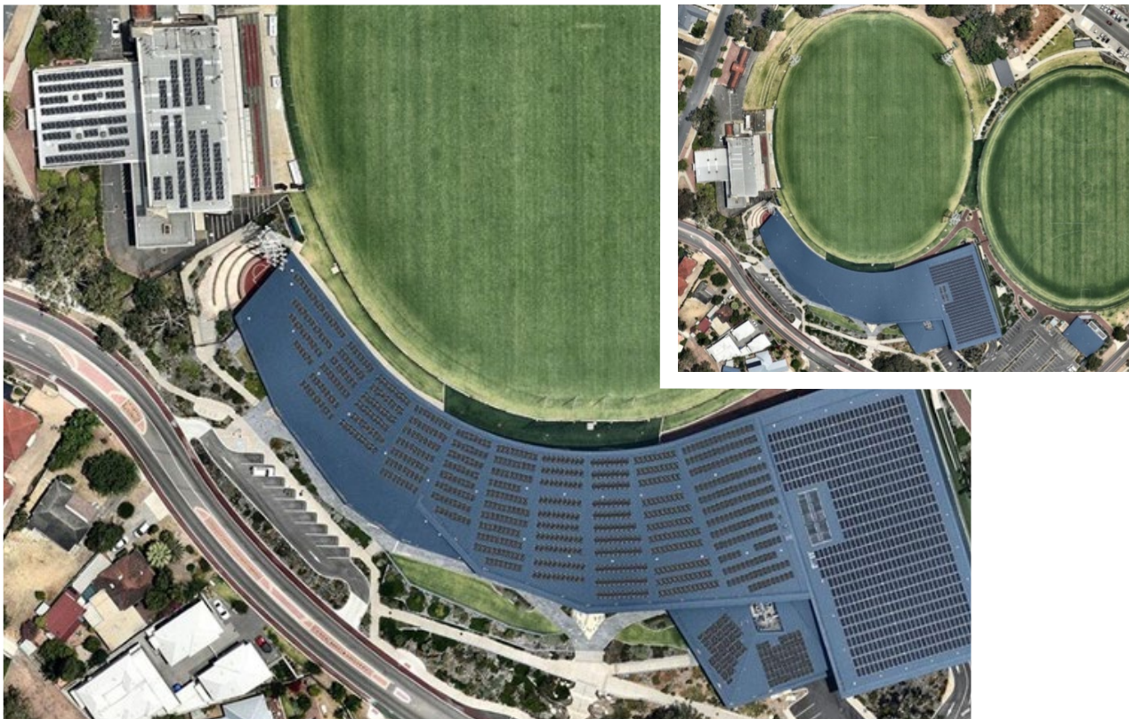
Figure 24: Mineral Resources Park, with existing solar system (inset) and with a potential additional 484 kW solar array
