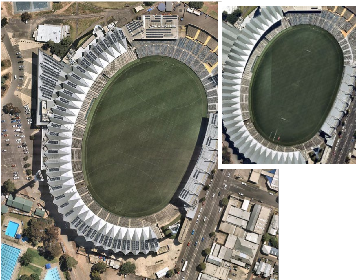
Figure 9: GMHBA Stadium, now (inset) and with a potential 559 kW solar array
