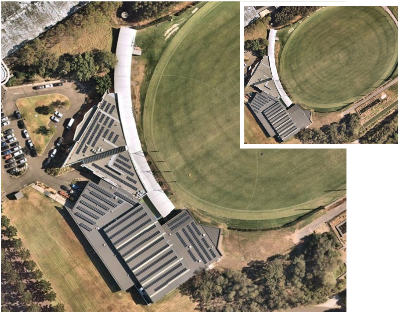
Figure 14: The Westconnex Centre, with existing solar system (inset) and with an additional 94 kW solar array
