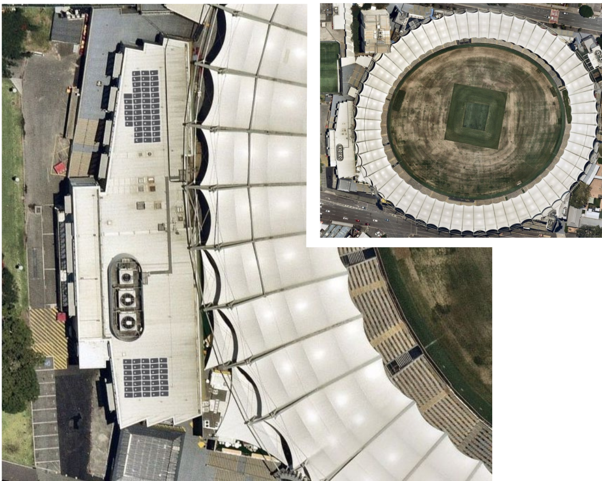
Figure 4: The Gabba, now (inset) and with a potential 28.8 kW solar array
