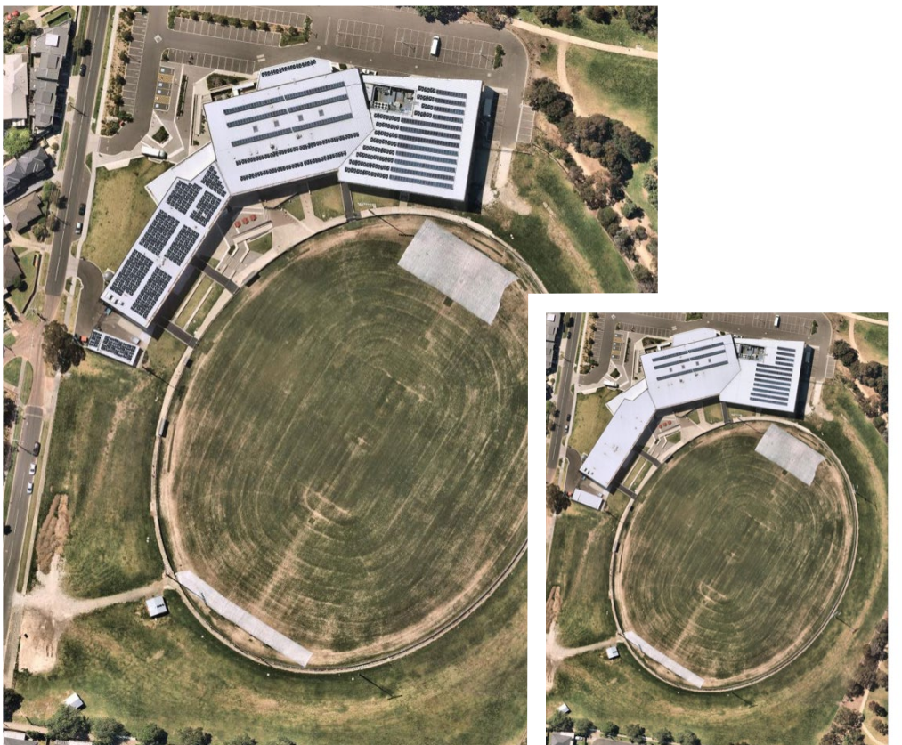
Figure 22: Moorabbin Oval, with existing 100 kW solar array (inset) and with potential additional 229 kW solar array
