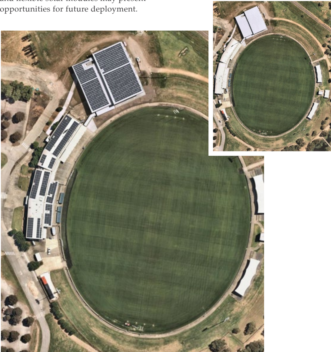
Figure 18: Casey Fields, now (inset) and with a potential 378 kW solar array
