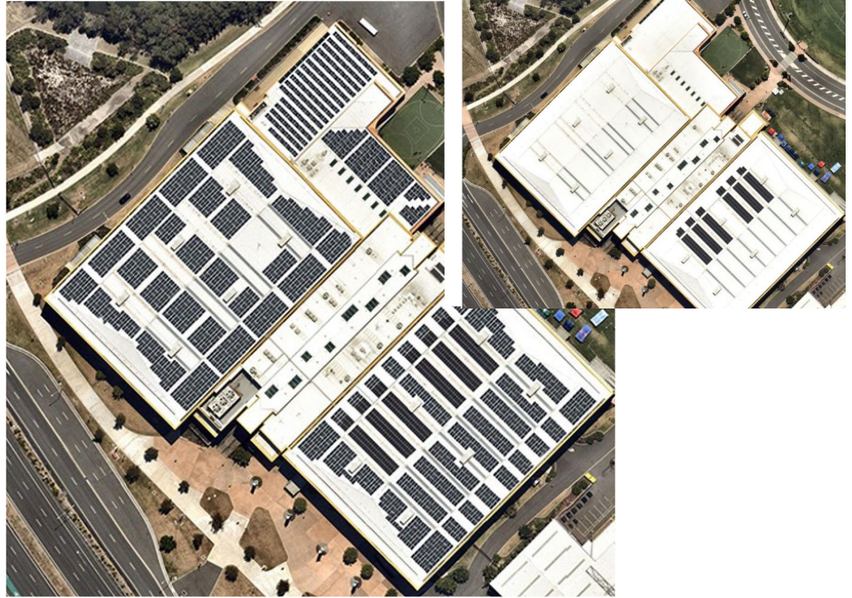
Figure 11: The Gold Coast Leisure Centre, with existing solar system (inset) and with potential additional solar arrays
