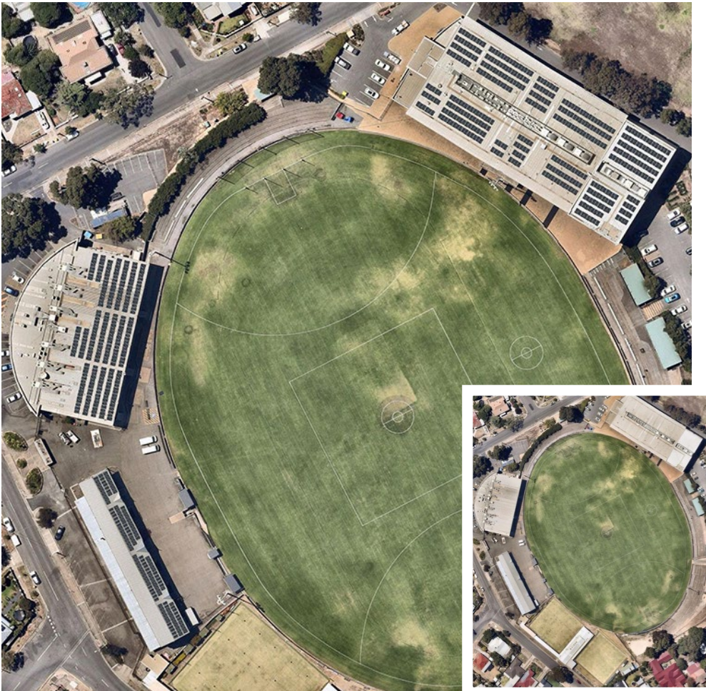
Figure 20: Alberton Oval, now (inset) and with a potential 301 kW solar array
