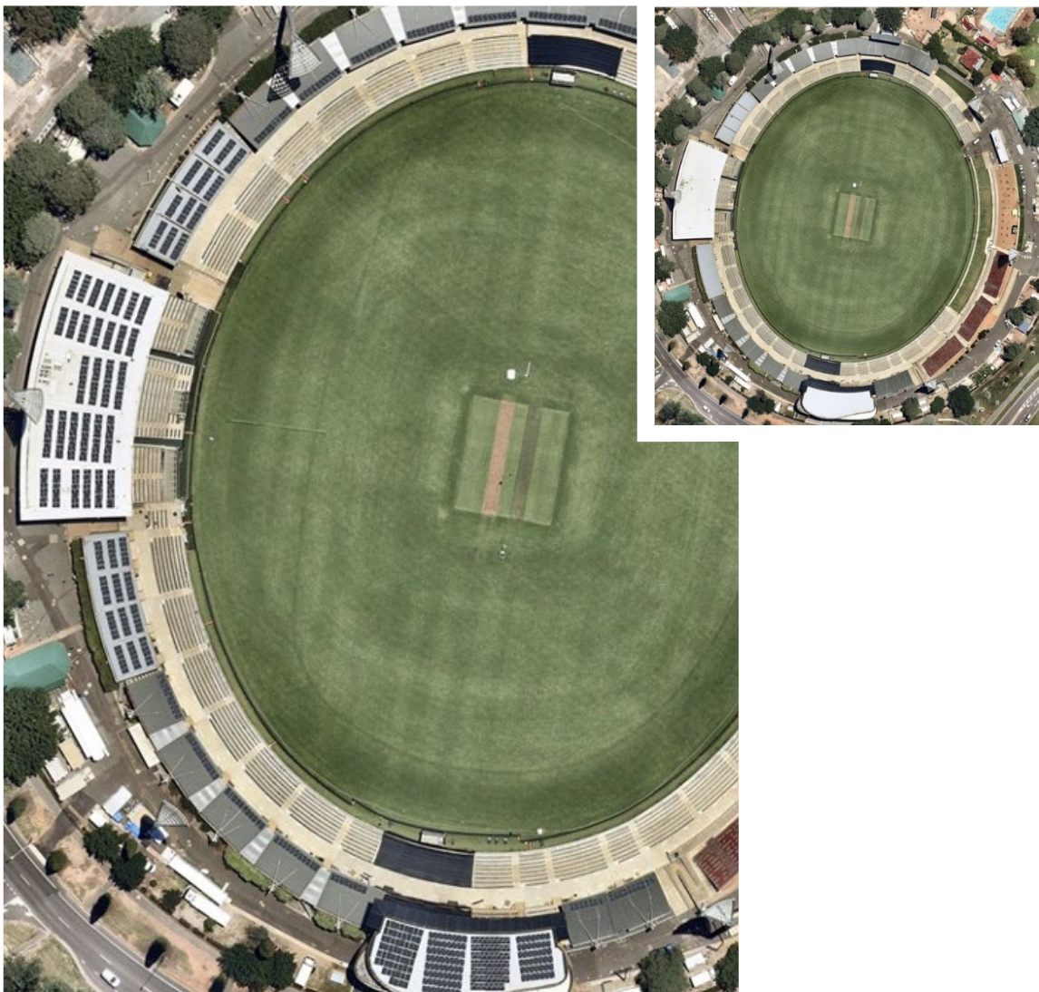
Figure 15: Manuka Oval, now (inset) and with a potential 269 kW solar array
