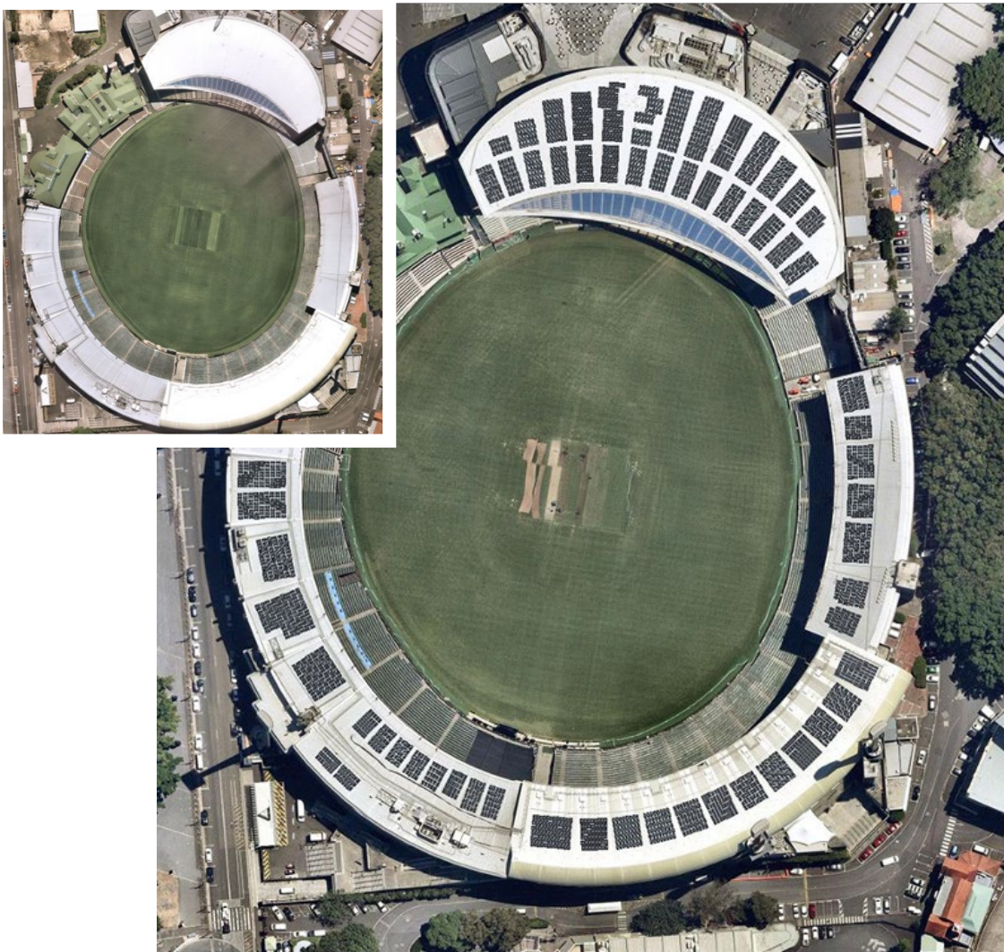
Figure 23: Sydney Cricket Ground, now (inset) and with a potential 1,004 kW solar array
